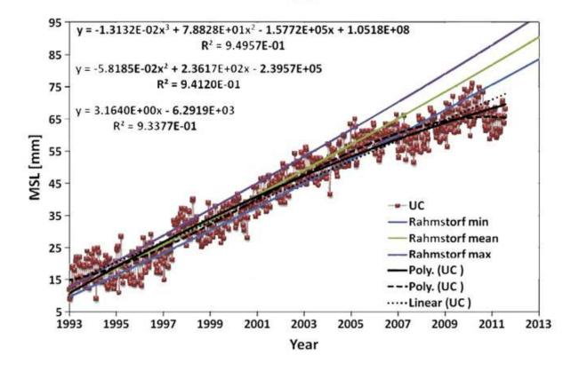
Figure 7. Comparison of Mean Sea Level (MSL) predictions from Rahmstorf (2007) with measurements from the TOPEX and Jason series. Adapted from Boretti (2012), who states in the figure caption that "the model predictions [of Rahmstorf (2007)] clearly do not agree with the experimental evidence in the short term."
